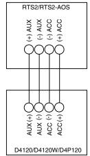
NOTE: If polarity of Acc. (+) and Acc. (—) are reversed, an Amber LED on sensor 2 of the duct smoke detector power board will exist indicating a trouble condition.
